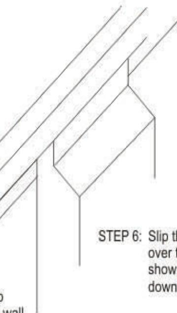
STEP 6: Slip the "J" channel over the pads as shown and secure it down in the "Z" channel.
